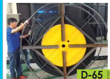
▲ Sabin Chain applied to winding equipment for long stroke cable chain
